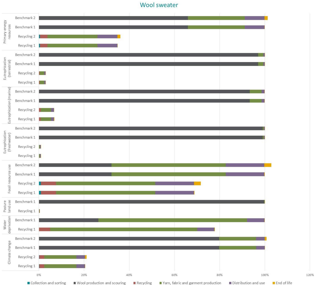
Figure 16. Results of case study D, for the recycling scenarios with 100% recycled input materials, and the benchmark scenarios with 100% primary input materials, and sub-scenarios 1 (incineration at end-of-life) and 2 (recycling after end-of-life). Results are normalised to benchmark scenario 1.
