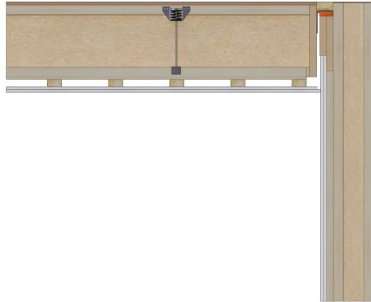
**Figure 7 Sectional drawing of the system showing mounting brackets and spring connections**
