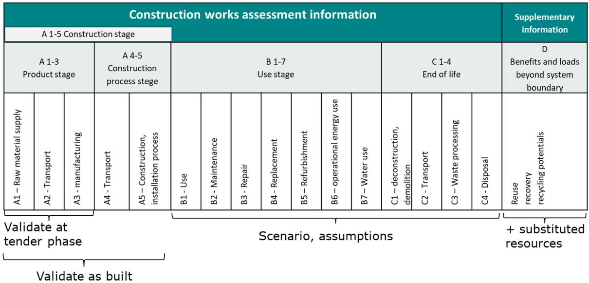
**Figure 4** The life cycle of a building divided into stages and information modules (EN 15804, EN 15978). "X" indicates stages in the life cycle included in the building system calculations reported here. In the Swedish translation of, SIS has introduced the name Construction Stage for module A1-5 (SIS 2020).
