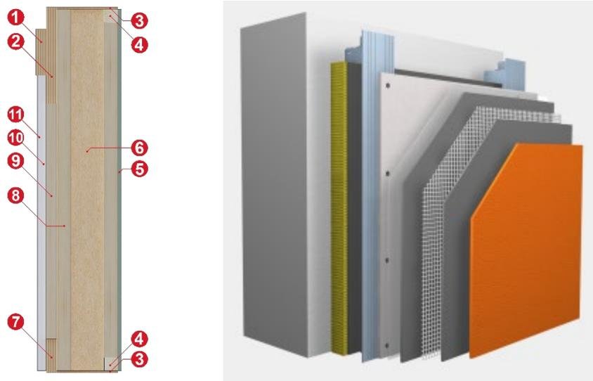
**Figur 6** Exterior wall construction up to exterior panel ; 1) LVL 33 mm, 2# LVL 33 mm, 3) hardboard 6 mm, 4) blockings 45 x 45, between Masonite studs, 5) Fermacell 12,5 mm, 6) Insulation, 7) LVL 33 mm, 8) R200, c600 + 195 mm Termoträ, 9) 34x95 c600 + 45 mm Termoträ, 10) Fermacell fire panel 15 mm, 11) Fermacell 12.5 mm.
