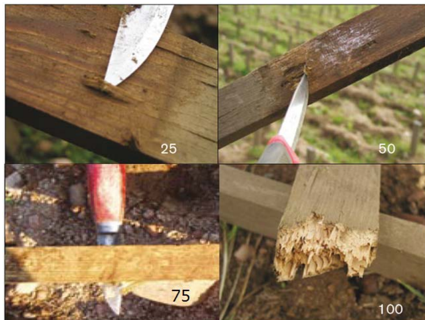
Figure 6 Visualisation of the decay index, in compliance with the European field testing standard EN 252, used for timber in ground contact. (Reference: Råberg, Terziev 2006)
