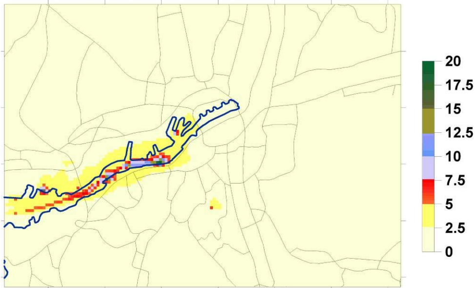
Figure 42. Total SO 2 concentration (µg/m 3 ) calculated with TAPM. The blue line indicates the main part of the harbour.
