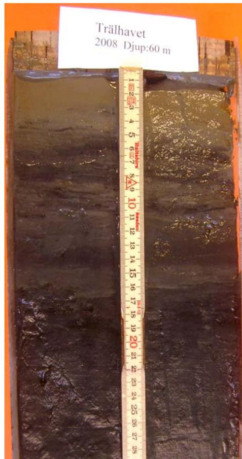
**Figure 1-21** A sediment core from Trälhavet Bay sampled in 2008 at a depth of 60 m.
