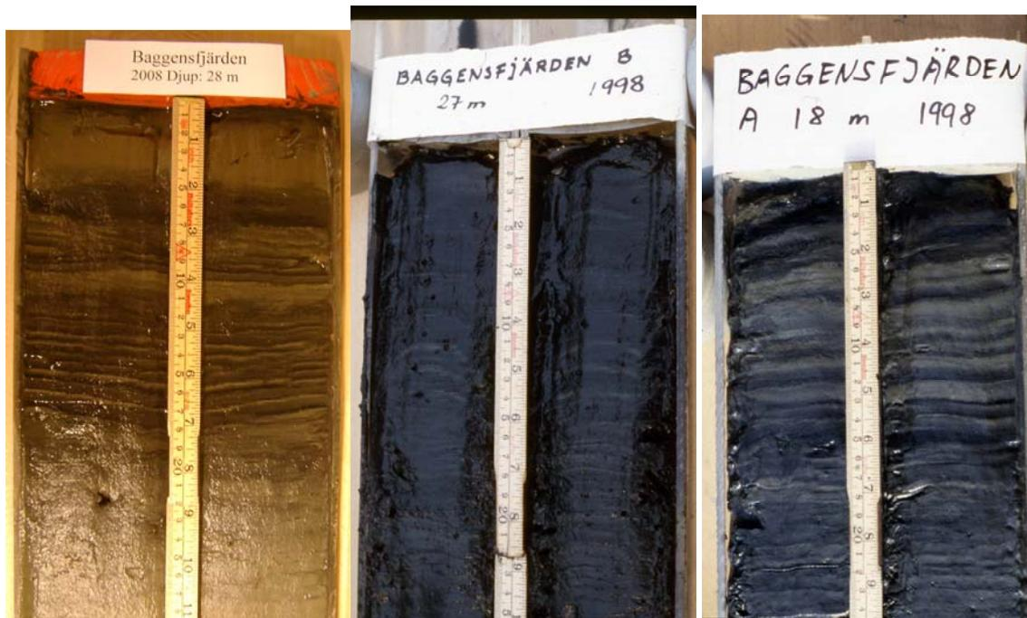
**Figure 1-19** Photographs of sediment cores from Baggensfjärden Bay from left to right 1/ 2008 depth 28 m, 2/ 1998 depth 27 m, 3/ 1998 depth 18 m.
