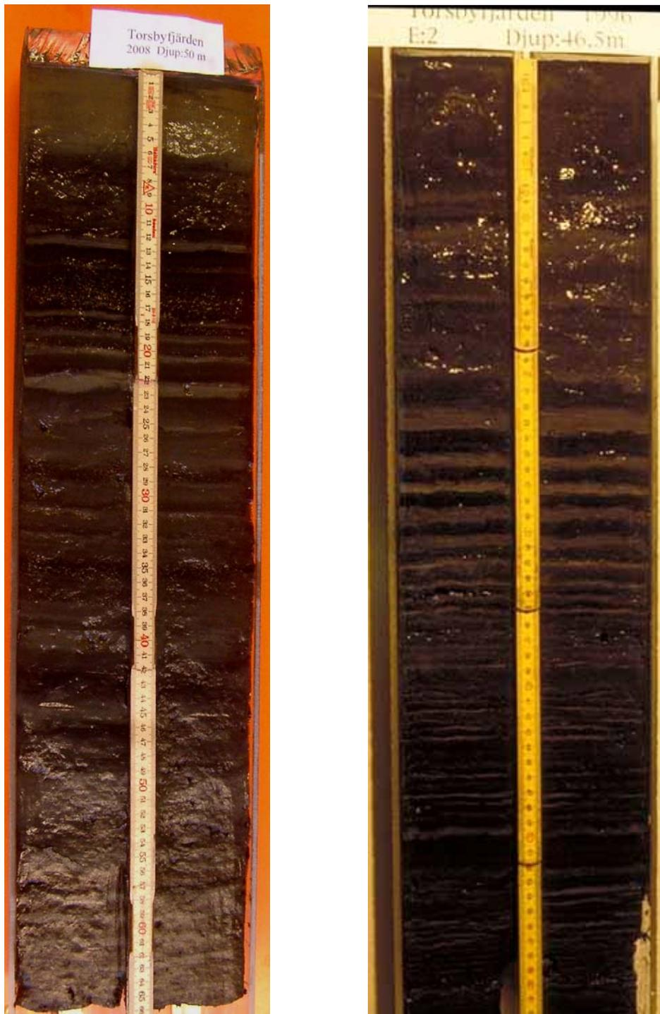
**Figure 1-16** Photographs of sediment cores from Torsbyfjärden Bay from left to right 1/ 2008 depth 50 m, 2/ 1996 depth 46.5 m.
