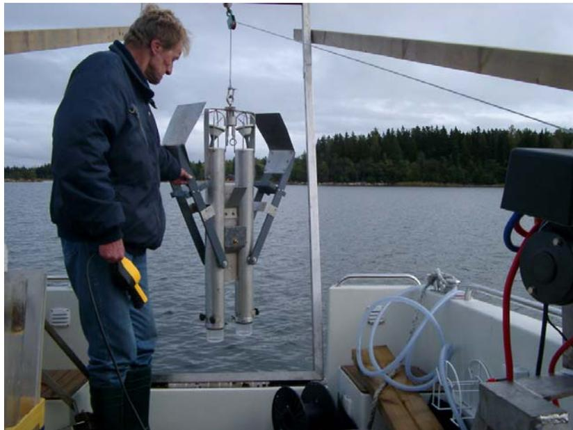
**Figure 1-12** The Gemini core sampler ready to be launched from Research Vessel Perca.
