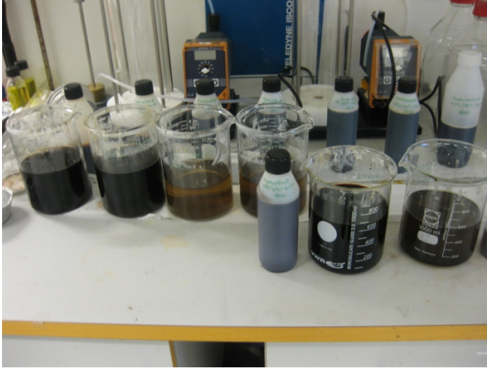
Figure 2: Third step, sedimentation, and plastic bottles containing the first supernatant removed.
