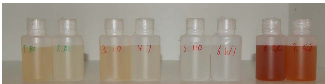
Figure 21 Water extract before (left) and after (right) photo catalytic processing. From left to right in the picture: B1, I1, W2, K20.
