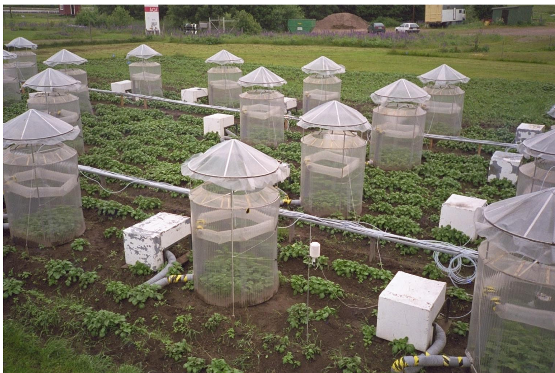
Figure 4-5 Open-top chambers used for crop research at Östad.
