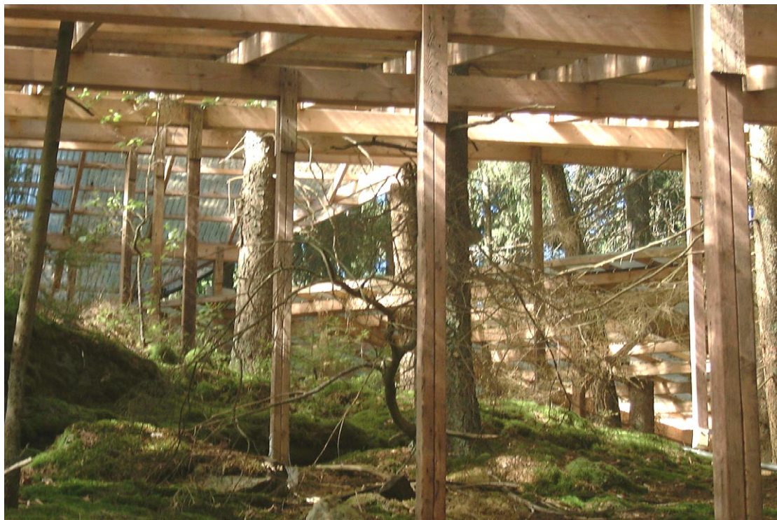
Figure 4-1 The Roof Experiment at Gårdsjön. View from under the roof.
