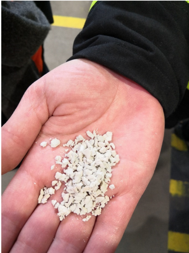
Figure 8. PVC granulate to be recycled into new Tarkett flooring in Ronneby
