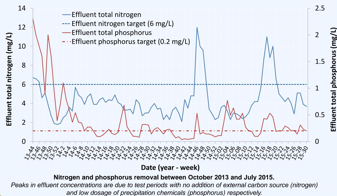
The process operation has been stable with a significant better capacity than expected. The process reaches preng/L defined effluent targets for nitrogen (6 mg/L) and phosphorus (0.2 mg/L), even at high loads. There is also a high removal of suspended solids (<1 mg/L).
